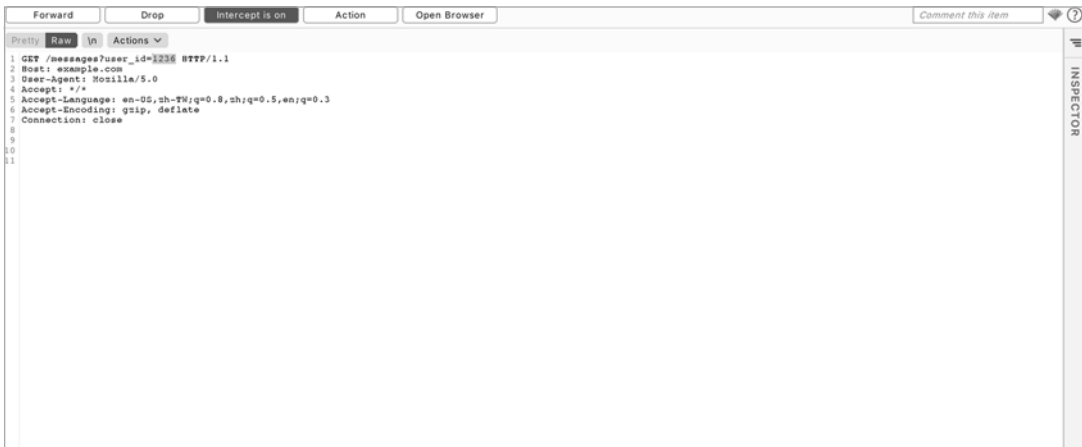
Figure 10-1: Modify the request in Burp's proxy window to switch out the IDs.
