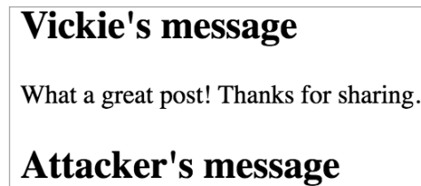
Figure 6-5: The HTML page with two messages rendered in the browser. You can see that the attacker's message is blank because the browser interprets it as a script instead of text.
