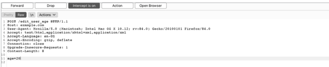
Figure 6-6: Intercept the outgoing request to edit it before relaying it to the server.
