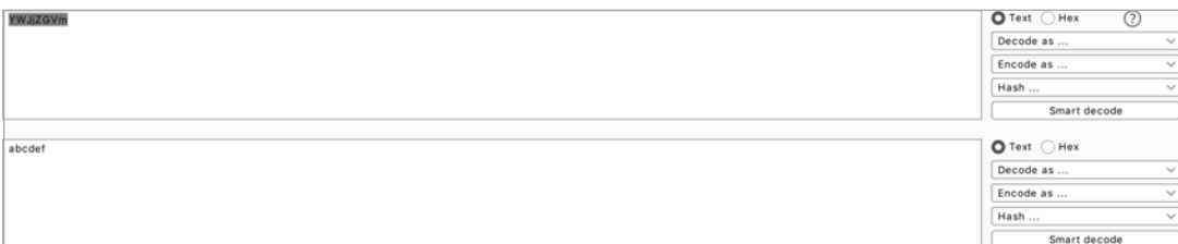
Figure 10-2: You can try to use different methods to decode a string in Burp's decoder. Or you can use the Smart Decode tool and see if Burp can detect the encoding scheme.
