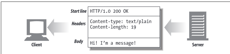
Figure 3-3. Three parts of an HTTP message
