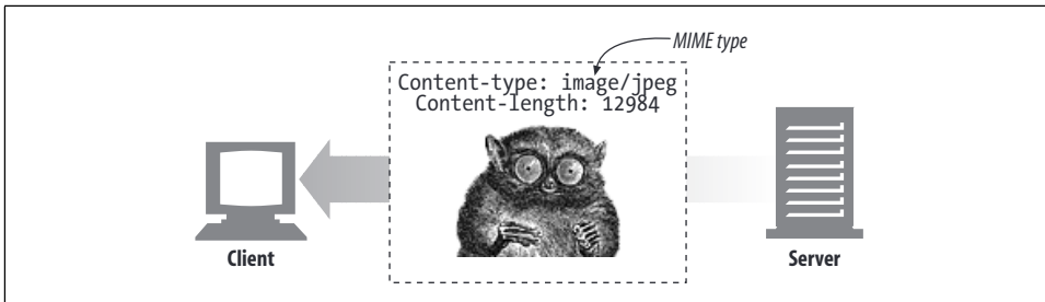
Figure 1-3. MIME types are sent back with the data content
