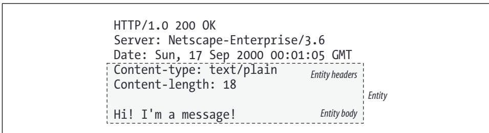
Figure 15-1. Message entity is made up of entity headers and entity body
