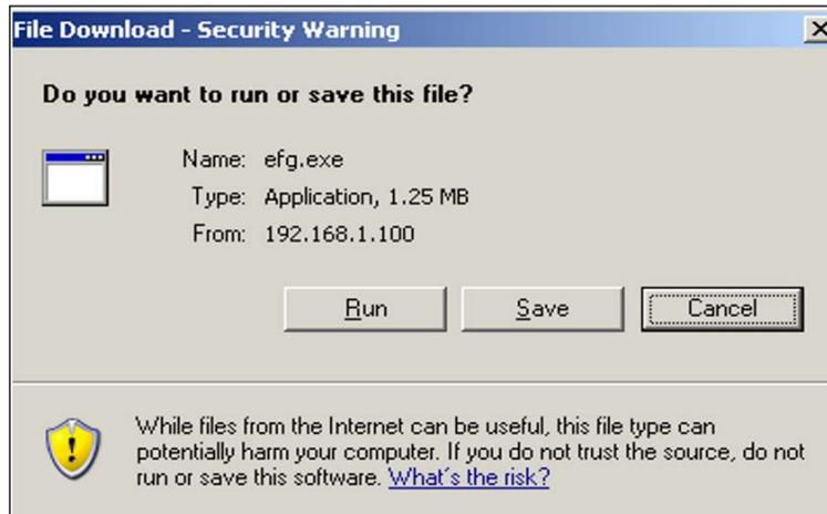
Figure 7.19: Client gets redirected to IP 192.168.1.100 and is asked to run the application.
