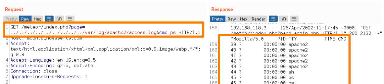
Figure 130: Output of the specified ls command through Log Poisoning
