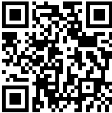
Figure 13.8 A QR code is a way to encode a URI that can be easily scanned by a mobile phone with a camera. This can be used to display the verification URI used in the OAuth2 device authorization grant. If you scan this QR code on your phone, it will take you to the home page for this book.
